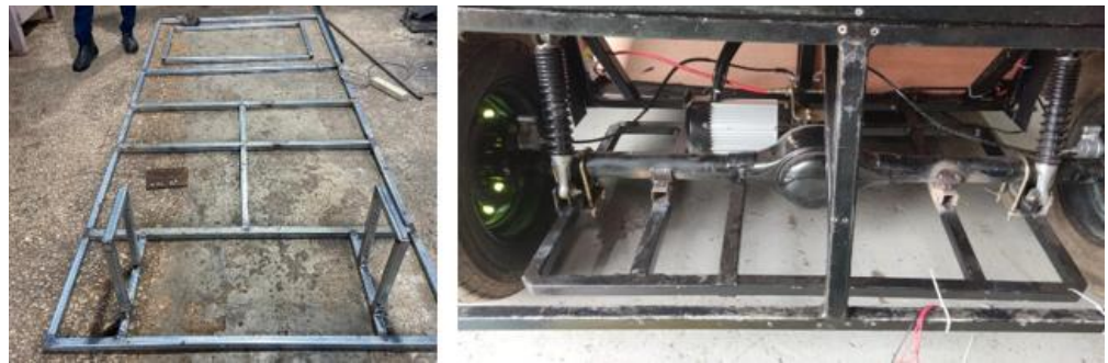
Gambar 1. Proses Fabrikasi ( Cutting, Welding, dan Grinding )
