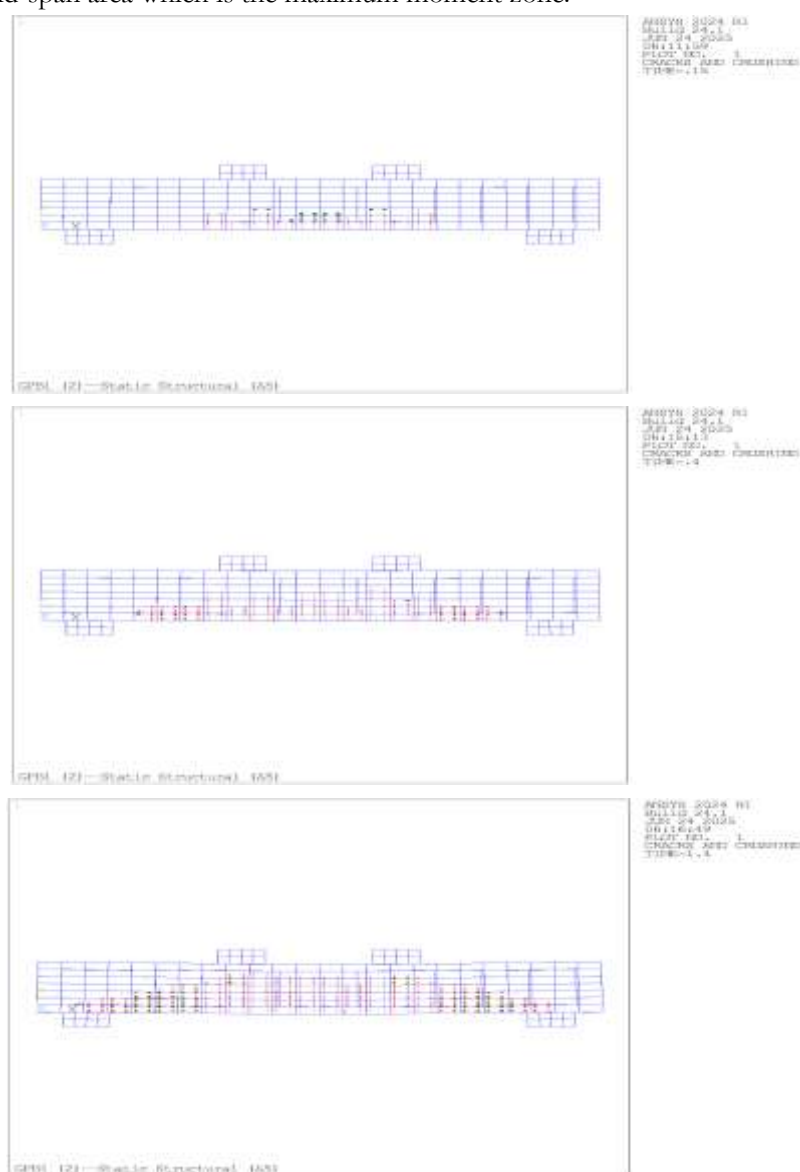
Figure 3. Crack propagation simulation of RGB1 beam (FEM)-ANSYS) based on experiments Abraham, et. al. 2013
