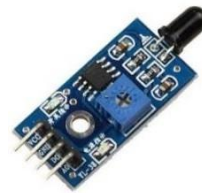
Figure 2. Fire Sensor (Source: arduinoindonesia.id).
