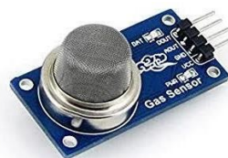
Figure 3. MQ-2 Gas Sensor (Source: andalanelektro.id).
