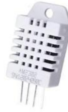
Figure 4. DHT22 Temperature Sensor (Source: core-elektronics.com).
