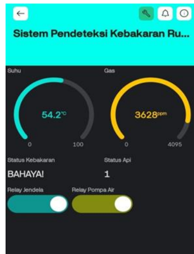
Figure 21. Display Condition Danger Detected Fire And Smoke/Gas.
