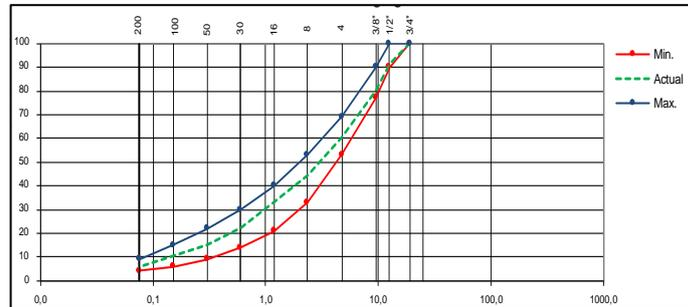
**Figure 1.** Laston AC-WC Aggregate Combination Chart.
