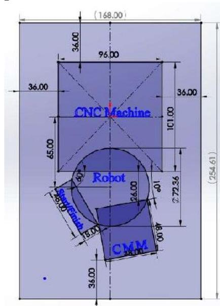
Figure 6: Plan of Industrial Cells
