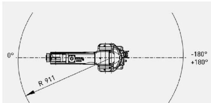
**Figure 2: Robot Rotation**
