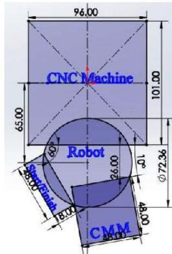
Figure 5: Collaborative unit Floor Plan
