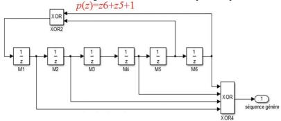
Gambar 2. Diagram sirkuit LFSR 6-bit
