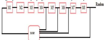
Gambar 4. Diagram sirkuit LFSR 8-bit
