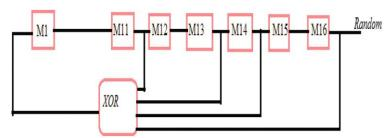
Gambar 5. Diagram sirkuit LFSR 16-bit
