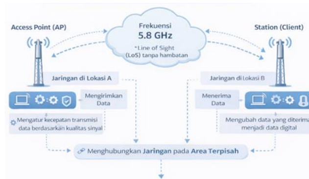
Gambar 7. Sistem Kerja Radio Wireless PTP 5.8 GHz
