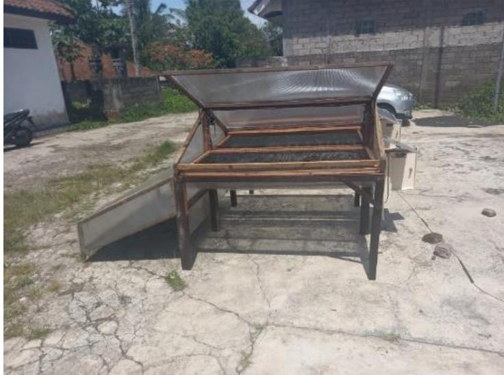
**Gambar 6.** Alat Solar Dryer Modular
